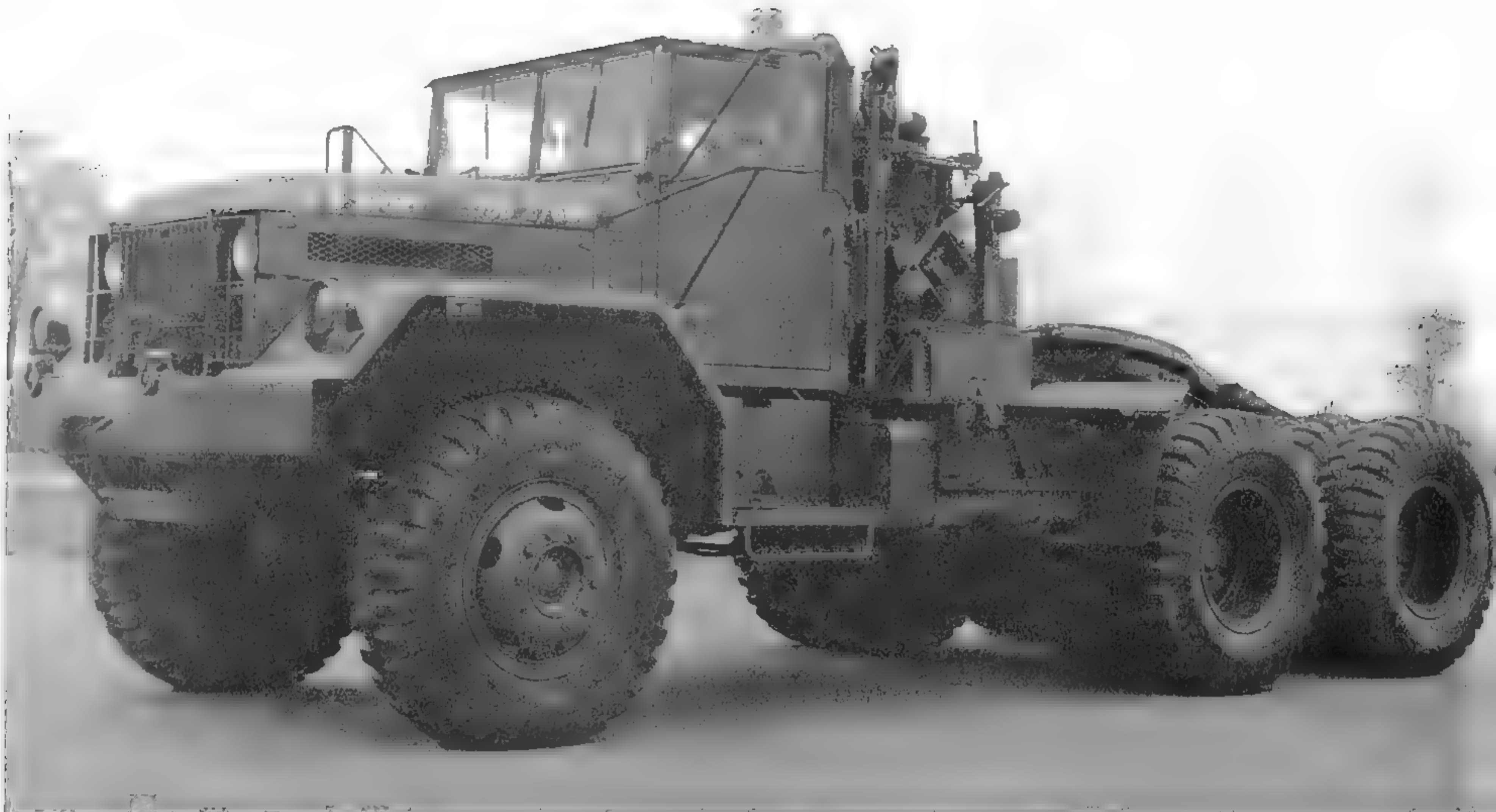
The dual winch-equipped M123E2 was powered by the V8-300 Cummins diesel engine. In addition to the clearance lamp mounted above the front tire, the M123E2 also had rearward-facing turn signal lamps mounted on the rear slope of the front fenders. Finally, the M123E2 was the first vehicle in this series to come equipped with a warning beacon. This amber beacon was mounted on the winch. (U.S. Army photo)
